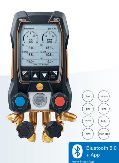
The testo 557s digital manifold with 4-way valve block enables you to carry out your measurements on refrigeration and air conditioning systems and heat pumps particularly fast. The large display also helps you to evaluate the results in graphic form. Stored programs guide you through the measurement and enable the automatic determination of numerous important system parameters such as superheat, pressure drop test or evacuation.
